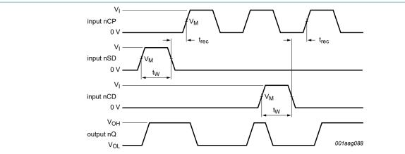
Recovery times are shown as positive values but may be specified as negative values. Logic levels:  $V_{OL}$  and  $V_{OH}$  are typical output voltage levels that occur with the output load. Measurement points are given in <u>Table 9</u>.
