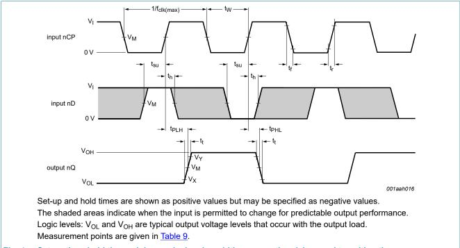
Fig. 4. Set-up time, hold time, minimum clock pulse width, propagation delays and transition times
